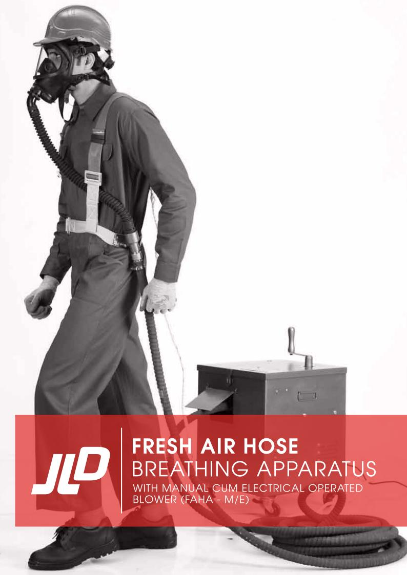
The JLD FRESH AIR HOSE APPARATUS consists of an ISI marked PROTECT 2000 Full Face Mask connected to a corrugated tube ending in a manifold mounted on a harness belt worn around the waist. The manifold is connected to a 15 meters long 20mm I.D. canvas covered wire-embedded rubber hose. The other end of the hose is connected to the electrical / hand operated blower.
